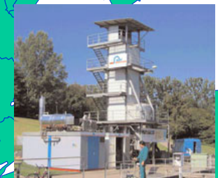
Gasification of Solid Sewage Residues
