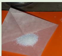
Zeolite 40-60 0.422 < D < 0.241 mm
