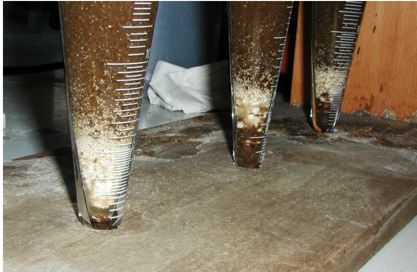
Figure 3: Precipitation by Ca(OH)_2 in RBW. From the picture it is possible to observe the precipitate in the bottom of the Imhoff cone.
