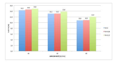
As expected, the higher amount of percentage increase of Kla and S.O.T.R. is obtained by fixing the liquid velocity and increasing the air velocity, while: if the airflow rate is fixed, the increase is very low. This means that: if an increase of Kla or S.O.T.R. is needed, the best thing to do is to increase the Air-side turbulence by increasing the AFR.
