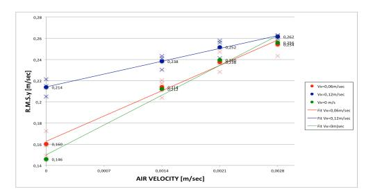
It can be noticed that the overall turbulence parameter increases linearly when the air velocity (and then the airflow rate) increases.
