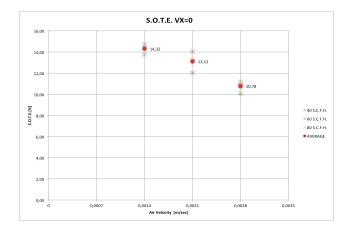
Both the volumetric mass transfer coefficient Kla and the standard oxygen transfer efficiency S.O.T.R. increase linearly (with different slopes) by increasing the air flow rate in the diffuser, while the S.O.T.E. has the opposite trend. This decrease is caused by several factors:
