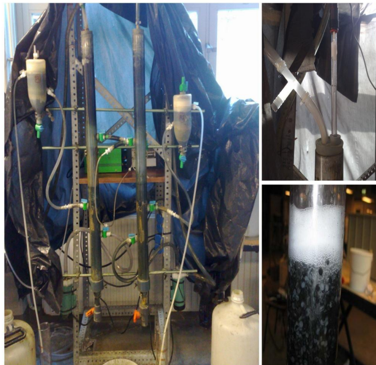
Figure 3.2 – IFBR's used in the lab, electrode used to measure and control the pH and example of turbulence of the bed.
